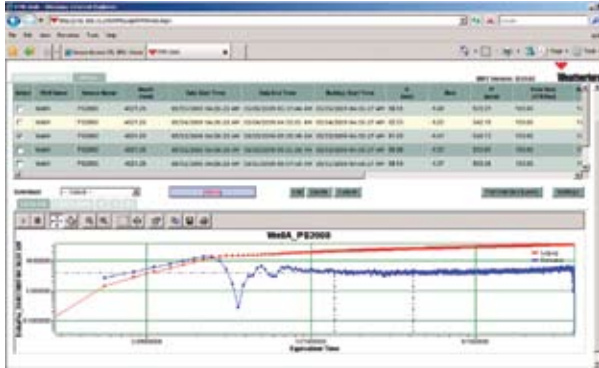
PanQL log-log plot: radial flow line and flow regime are fitted automatically to derive k and S . P^* is obtained from a Horner plot.
