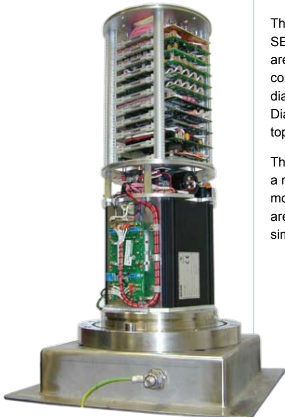
Subsea electronic module with open communication controller
