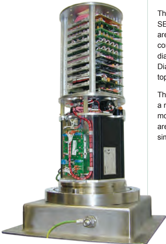
Subsea electronic module with open communication controller
